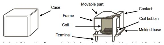
\* Please pay particular attention to special metals (alloys) used for plastic flame-retardants, and electrical characteristics and lubrication of contact points.
