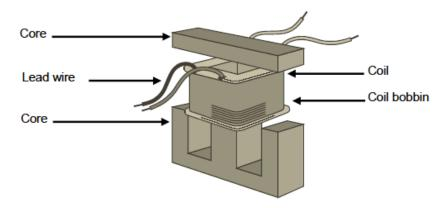
\*Please pay particular attention to flame retardants in plastic materials or insulating parts, inpregnant in the coil, PVCs or flame retardants in the lead wire.
