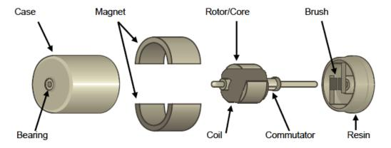
\*Please pay particular attention to special metals (alloys) used for flame retardants in plastic, and electrical characteristics and lubrication in commentators, as well as grease in bearings.
