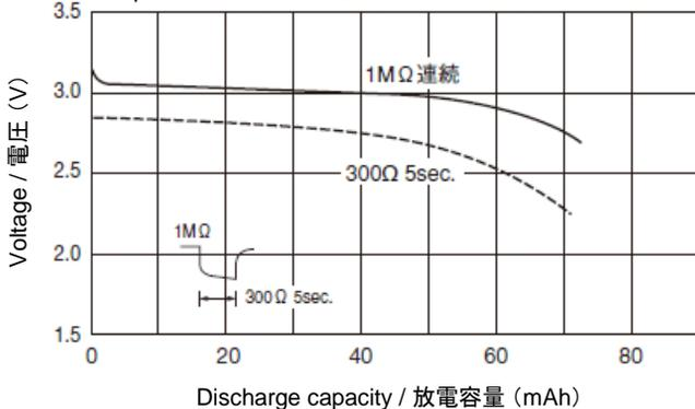
Discharge Load vs. Discharge Capacity of CR2016
