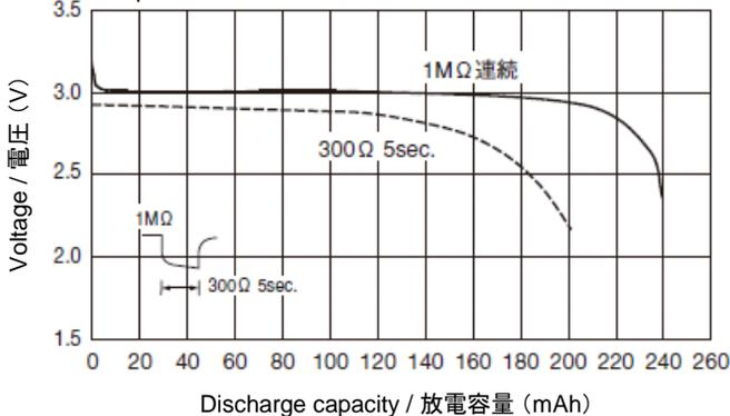
Discharge Load vs. Discharge Capacity of CR2032
